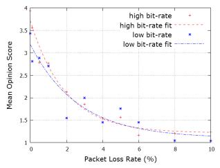
Figure 5. Fitting curve of subjective 3D quality vs Network loss
