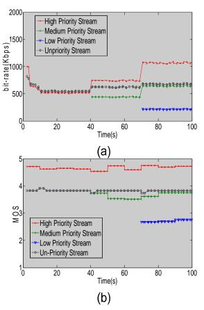
Fig.8. a) Bit-rate variation of equal priority scheme as a function of time b) Variation of the estimated user perceived quality expressed in terms of MOS when considering the GOP structure of traffic traces
