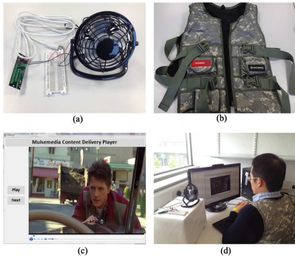
Fig. 2. Equipment and software used in the mulsemmedia delivery system employed in the user tests. (a) USB fan. (b) Haptic vest. (c) Player. (d) Test-bed.
